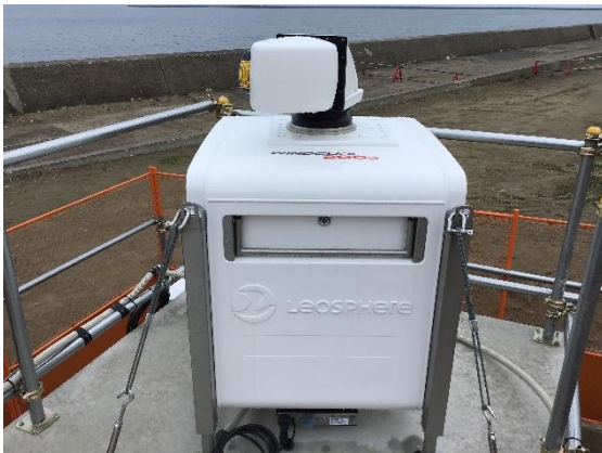
Wind conditions survey (Wind condition measurements using scanning LiDAR)
